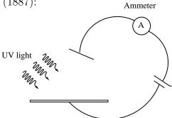
Polished metal plates emit electrons when irradiated by UV light. Energy of EM wave apparently liberates electrons.
