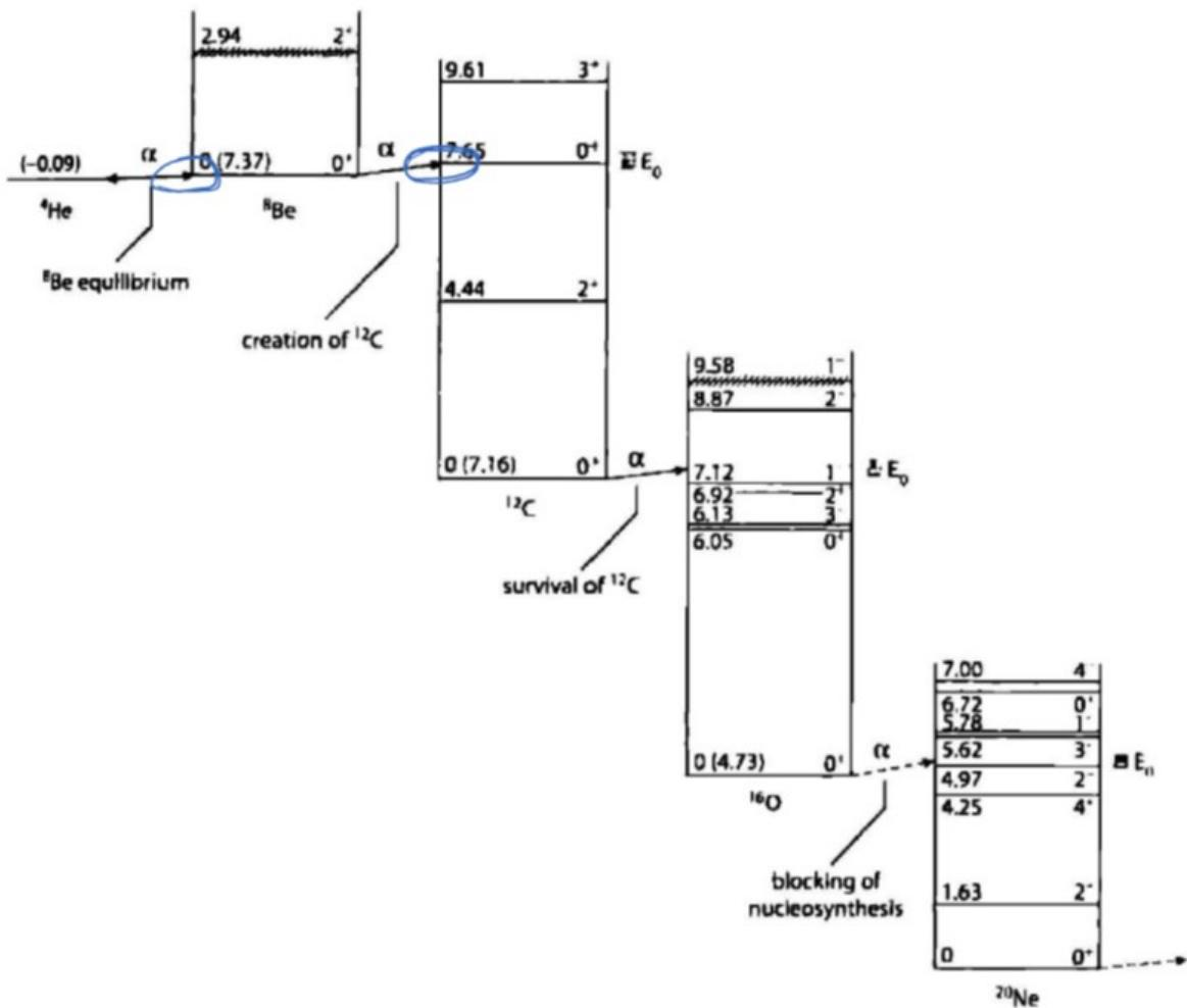
Figure 12.11 Energy levels of nuclei participating in thermonuclear reactions during the helium burning stage in red giant stars (adapted from [RR88]). The survival of both  $^{12}\text{C}$  and  $^{16}\text{O}$  in red giants, believed to be the source of terrestrial abundances depends upon fortuitous circumstances of nuclear level structures and other properties in these nuclei.
