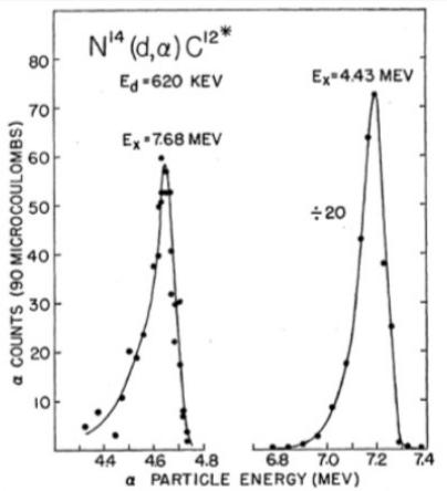
FIG. 1. Alpha spectrum from  $\text{N}^{14}(d,\alpha)\text{C}^{12}$  obtained with a thick  $\text{NH}_3$  target. No other groups were observed in the range  $E_\alpha = 3.7 - 7.4$  Mev of magnitude 1 percent of the group to the 4.43-Mev state. The spectrometer was set at  $\theta_{lab} = 90^\circ$ .
